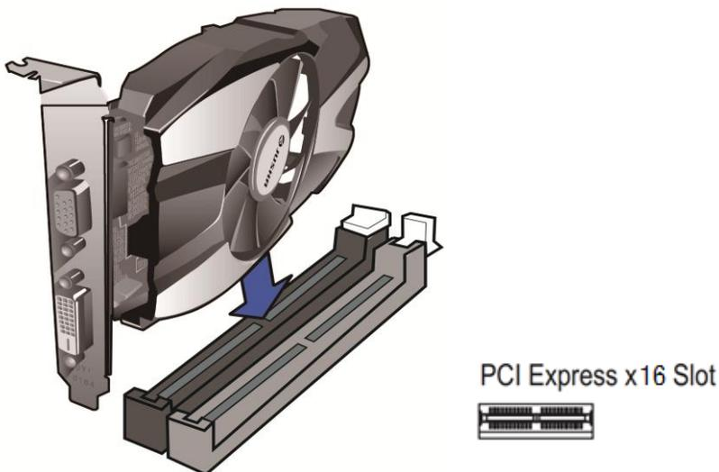
4. Secure the card's metal bracket to the chassis back panel with a screw.
