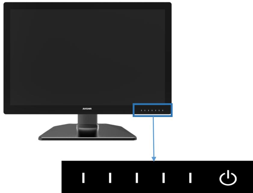
The keys except power key are silkscreen keys. Press any key except power key to bring up the navigation key icons, as shown below.
